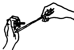
B-17 Improper way to insert glass tubing in a stopper.
