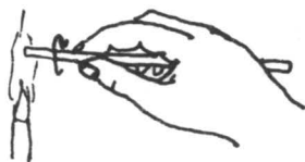
B-4 Fire polishing (note rotation of the work)
